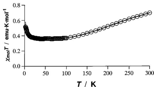
**Figure 7.** Temperature dependence of  $\chi_{\text{mol}}T$  of triradical **N** at a constant field of 5000 Oe. The solid curve is the theoretical one described in text.
