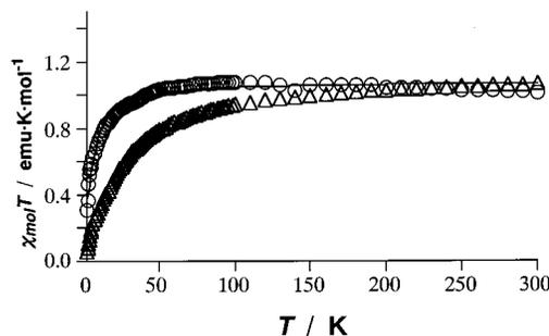
**Figure 10.** Temperature dependence of  $\chi_{\text{mol}}T$  of triradical **B'** in neat crystals ( $\Delta$ ) and 6% PVC film ( $O$ ) at a constant field of 5000 Oe. The solid curve is the theoretical one described in text.
