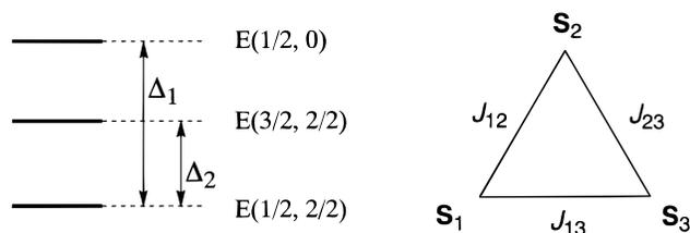
**Figure 8.** Energy level diagram for the two spin doublets and the spin quartet originating from the interaction of  $S_1 = S_2 = S_3 = 1/2$ .
