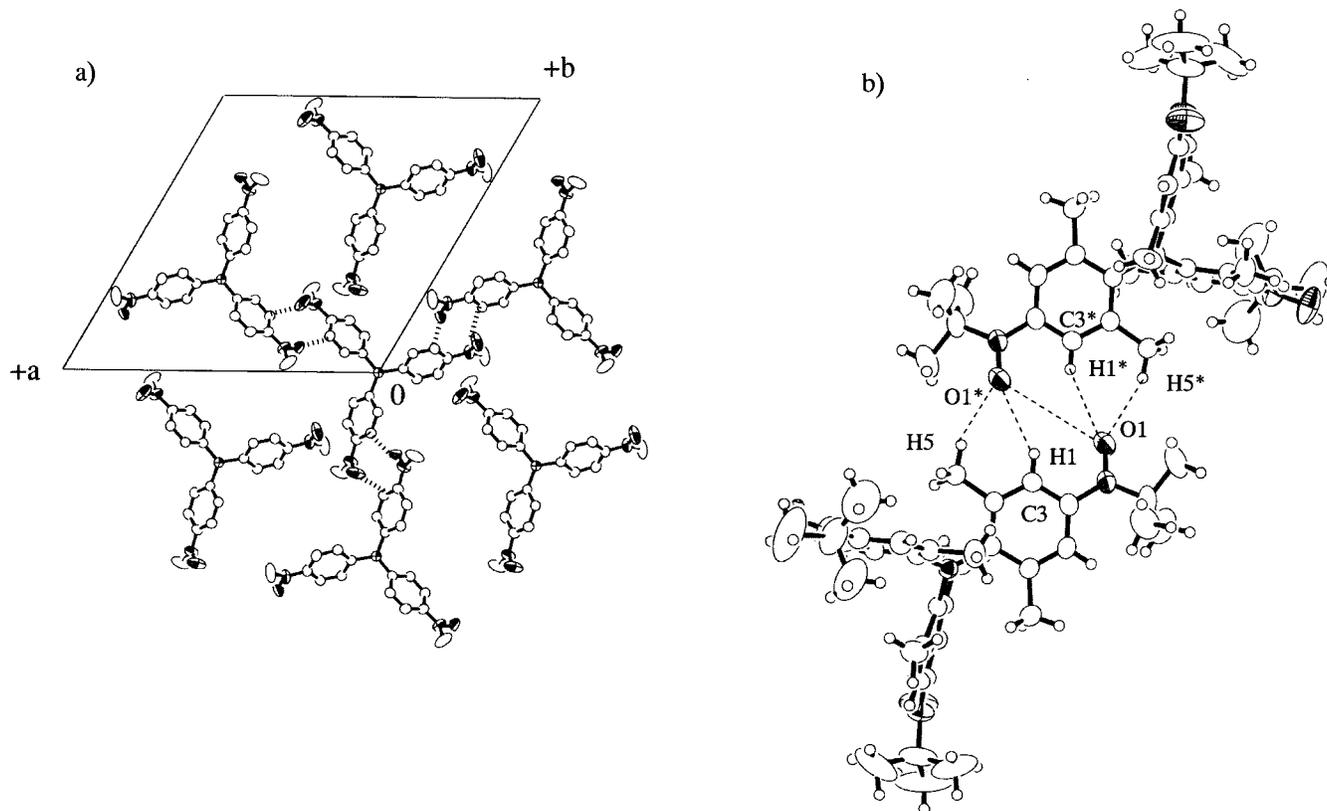
**Figure 5.** (a) Projection along the *c*-axis of **B'**. The methyl groups are omitted for clarity. (b) Crystal structures of **B'** in which the nearest molecules are shown. Broken lines indicate the short contacts between the neighboring molecules: O1–H1\* 2.66 Å, O1–O1\* 3.99 Å, O1–H5\* 2.45 Å.
