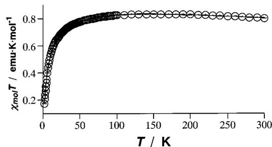
**Figure 9.** Temperature dependence of  $\chi_{\text{mol}}T$  of biradical **C** at a constant field of 5000 Oe. The solid curve is the theoretical one described in the text.
